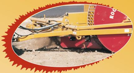
An optional drag plate can be installed when picking rocks on firm soil or in a pasture. The drag plate prevents rocks from being kicked forward onto previously picked ground.
