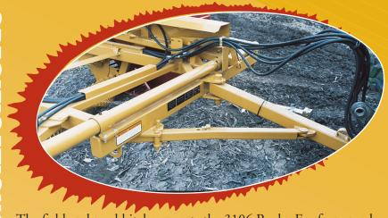
The field and road hitch converts the 3106 Rocke-Eze from road to field and back to road. The field and road hitch centers the 3106 behind the tractor for easier road transport.
