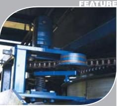
Single Drive Orbit Motor Heavy Duty 120H Chain 8" (20.32 cm) Heavy Duty Tub Channel Continuous Drive Sprocket Around Tub
