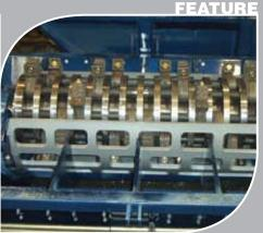
4 7/16" (11.27 cm) Bearings 7" (17.18 cm) Rotor Shaft 2" (5.08 cm)Hammer Rods 1" (2.54 cm) Replaceable Wear Plate
