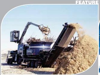
36" (91.44 cm) Wide Stacking & Belly Belts 25 Degree Oscillation Side To Side
