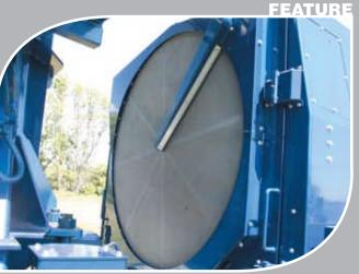
Self Cleaning Air Intake System Hydraulically Powered 3400 sq in (21,935.4 sq cm) Of Air Passage
