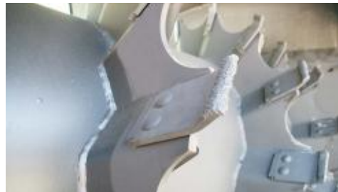
Additional hardening – armoured drum tools
