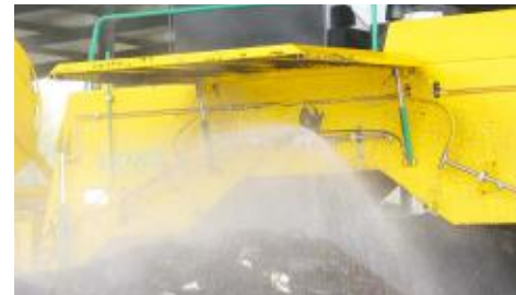
Process optimisation – injecting water during turning
