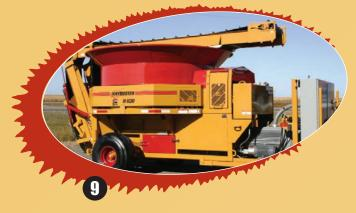
10. High-capacity grain grinding is another important operation that the H-1130 can also accomplish. By removing the mill grate/slug bar, placing the optional grain-grinding hopper over the hammermill opening and changing screens, the H-1130 becomes a high capacity grain grinder for grinding and/or cracking feed grains.
