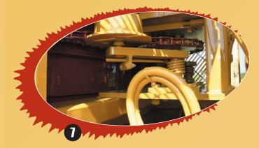
8. The H-1130's tub opens a full 90 degrees for easy access to the hammermill and drive train for daily maintenance and easy screen changing.
