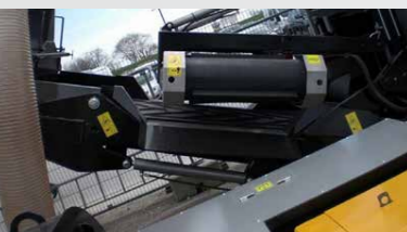
Hydraulic adjustable oberbelt magnet
