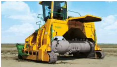
For increased traction on loose ground – the landfill undercarriage
