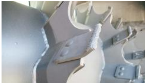
Additional hardening – armoured drum tools
