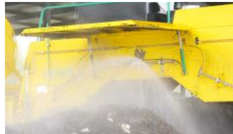
Process optimisation – injecting water during turning
