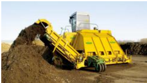
Intelligent space utilization – Side Conveyor
